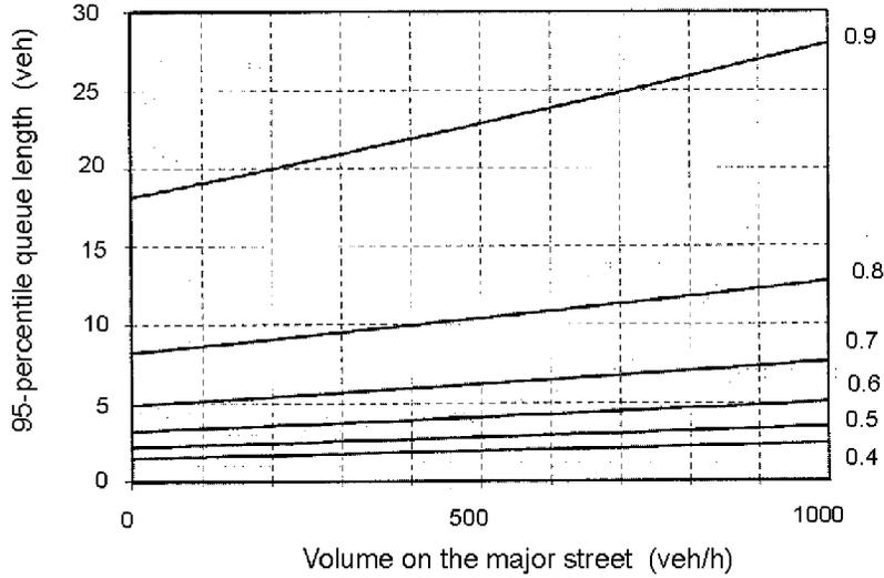
The parameter of the curves (indicated on the right side) is the degree of saturation ( $x$ ).
