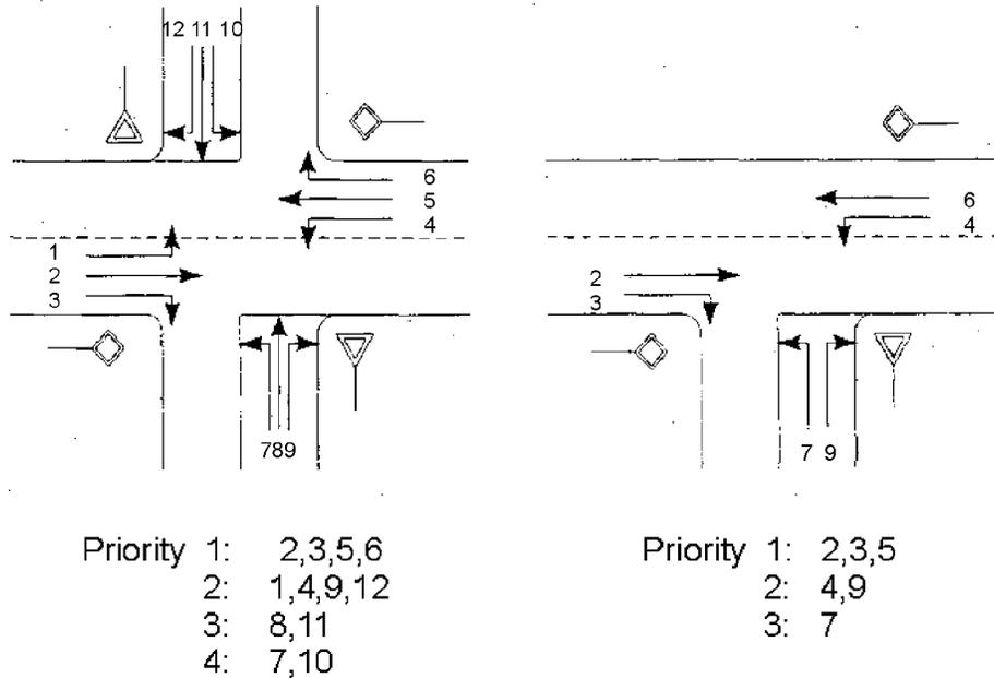
Note: The numbers beside the arrows indicate the enumeration of streams given by the Highway Capacity Manual (1994, Chapter 10).
