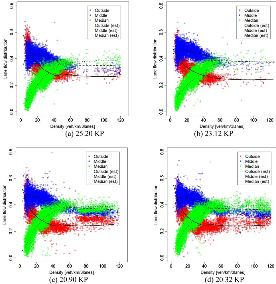
FIGURE 5. Comparisons between observations and estimations of lane flow distribution
