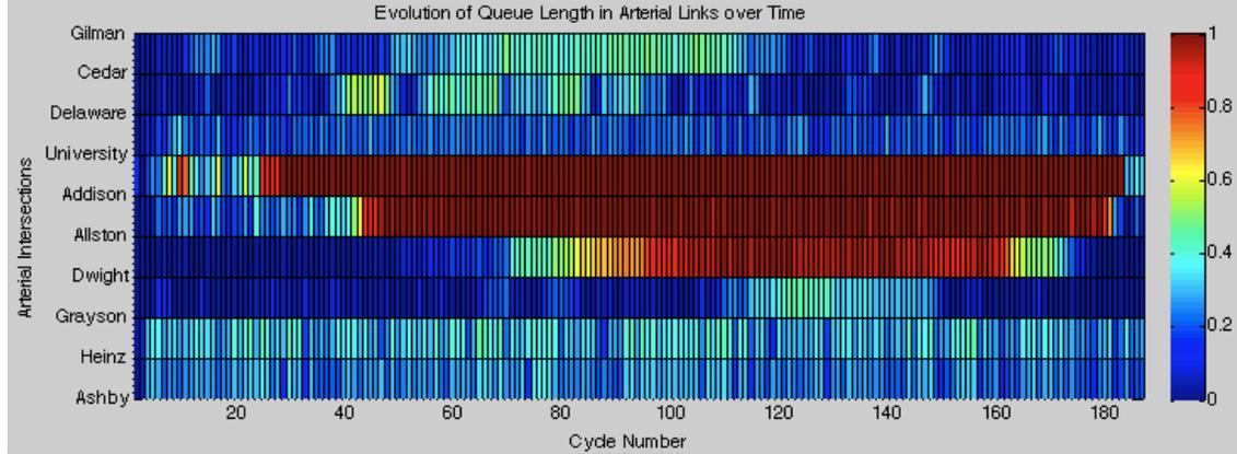
(b) Evolution of link queue lengths over time with fixed-time control (links queue occupancy from 0 to 1).
