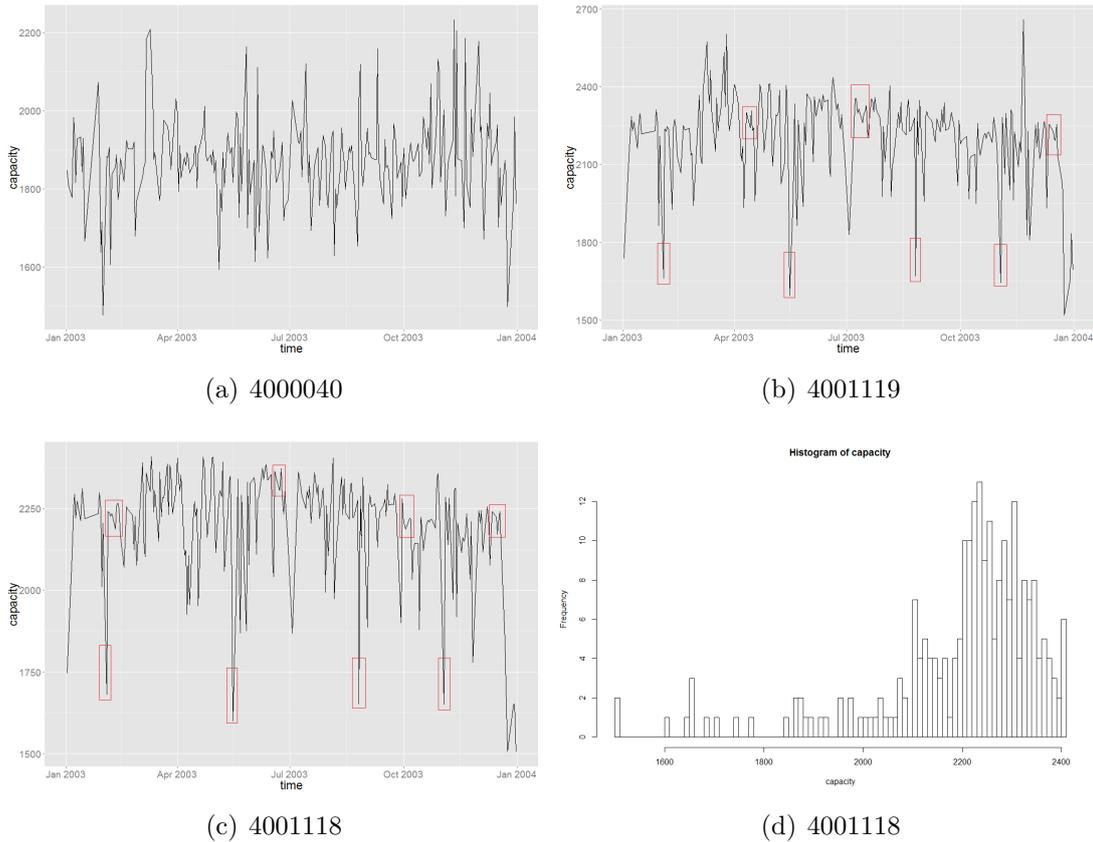
**FIGURE 1** Capacity variation patterns on basic freeway segment from multiple Georgia 400 detectors over a whole year's weekday observations
